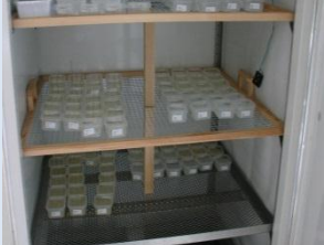
Climate chamber with a constant temperature of 12°C and a light period of 12 h (22,900 lux)
